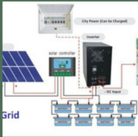
Off Grid Solar Power with battery bank
